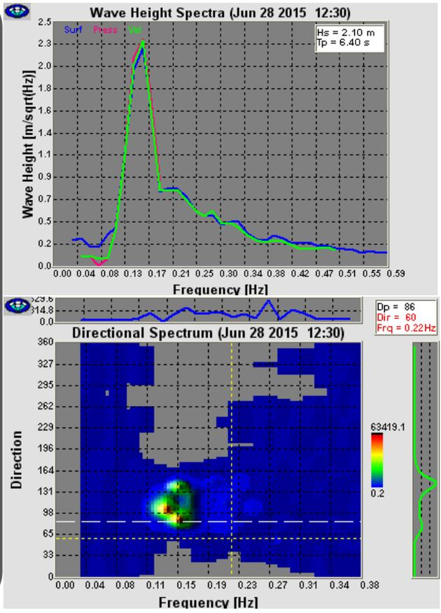
The wave data were a critical component of the overall project and were used to provide an understanding of wave propagation within the vicinity of Duxbury Beach, as well as to provide validation data for the numerical wave transformation model. A bottom-mounted Acoustic Doppler Current Profiler (ADCP) was deployed on May 14<sup>th</sup>, 2015 and measured directional waves, currents, and water depth for just over two months.
