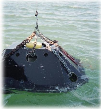
The ADCP system was deployed in a trawl resistant bottom mooring along with a pop-up buoy and an acoustic pinger to aid in the recovery of the mooring. The ADCP system was deployed just offshore Duxbury Beach (as shown on Page 3-3) in approximately 38 feet of water.
