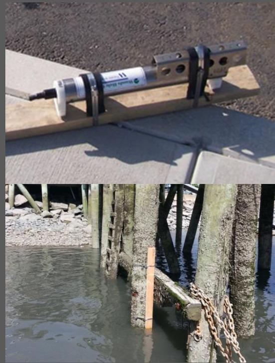
A Woods Hole Group Seapac 2100 tide gauge system. At the Harbormaster dock location, the instrument was securely fixed to a 2x4 and attached to one of the dock piles. By attaching the tide gauge to a 2x4, the instrument could be lowered deep enough to ensure the instrument would remain submerged for the entire tidal cycle. At the other locations (Clarks Island and Upper Marsh), the instruments were secured to a pipe anchor in driven into the seafloor.
