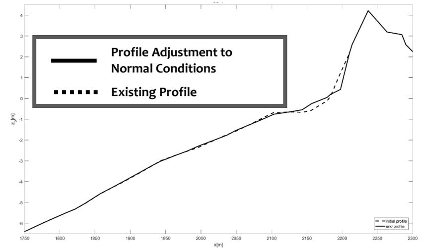
Response of the beach profile (showing cross-shore movement of sediment) fronting the Pavilion region for normal, average annual tidal and wave conditions. Minor erosion of lower dune face and beach berm.
