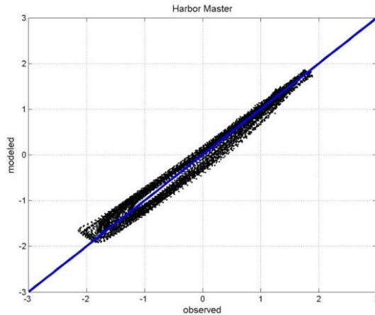
Statistical results of water surface elevations calibration.
