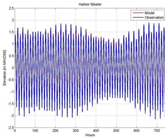
Visual comparison of the modeled water surface elevation results (red line) with the observed water surface elevation results (blue line) shows good agreement. This figure shows the comparison at the Harbormaster station. Water surface elevation is shown on the vertical axis (meters, NAVD88), while time is shown on the horizontal axis (hours).
